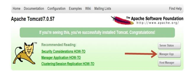
Deploy ETLValidatorServer.war file from datagaps server download using the deployment option in tomcat manager app as shown below :
